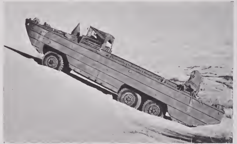
FIGURE 46. Desert tread tires, correctly deflated, enable DUKW to climb sandy hills. . . .
